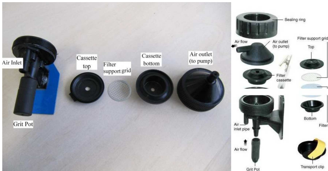
Figure 7. Casella (left) and SKC Ltd. (right) cyclones components
