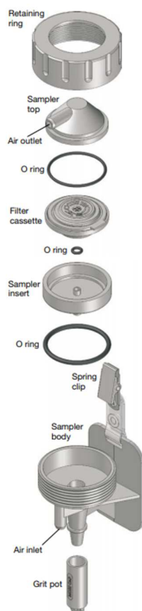
Figure 13. Configuration for plastic cyclone sampler and cassette
