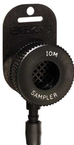
Figure 3. IOM conductive plastic sampler (Source: SKC. Inc)
