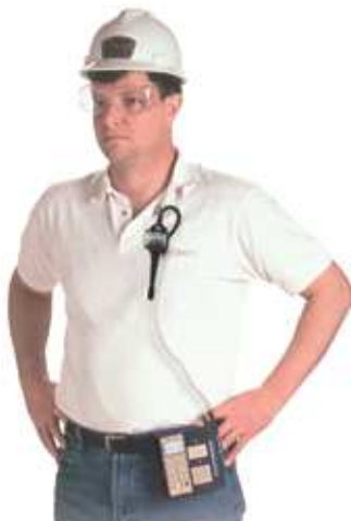
Figure 2. Illustration of sampler placed within breathing zone of worker, about 20-30 cm hemisphere around the nose and mouth (© Copyright 2018 SKC Inc.)
