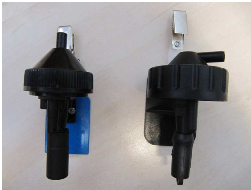
Figure 4. Higgins Dewell cyclone sampler (SKC on right, Casella on left)
