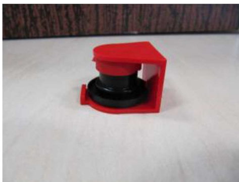
Figure 9. Loaded cassette with IOM cover awaiting to be labelled and used for sampling
